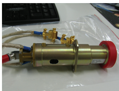
Euclid cold gas thruster, engineering model Selex ES
